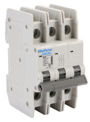
Gladiator miniature circuit breaker, 40A, 240 VAC / 125 VDC, 3-pole, B curve, thermal magnetic, 10kA @ 240 VAC interrupting rating, 35mm DIN rail mount.
