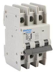
Gladiator miniature circuit breaker, 3A, 480Y / 277 VAC / 125 VDC, 3-pole, B curve, thermal magnetic, 10kA @ 480Y/277 VAC interrupting rating, 35mm DIN rail mount.
