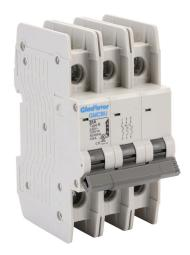
Gladiator miniature circuit breaker, 32A, 240 VAC / 125 VDC, 3-pole, B curve, thermal magnetic, 10kA @ 240 VAC interrupting rating, 35mm DIN rail mount.
