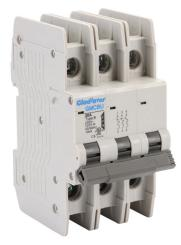
Gladiator miniature circuit breaker, 30A, 240 VAC / 125 VDC, 3-pole, B curve, thermal magnetic, 10kA @ 240 VAC interrupting rating, 35mm DIN rail mount.
