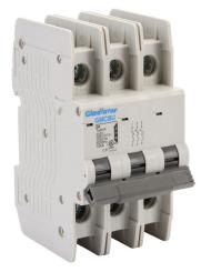
Gladiator miniature circuit breaker, 2A, 480Y / 277 VAC / 125 VDC, 3-pole, B curve, thermal magnetic, 10kA @ 480Y/277 VAC interrupting rating, 35mm DIN rail mount.
