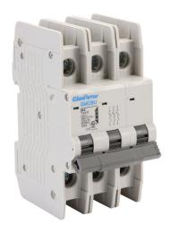
Gladiator miniature circuit breaker, 25A, 480Y / 277 VAC / 125 VDC, 3-pole, B curve, thermal magnetic, 10kA @ 480Y/277 VAC interrupting rating, 35mm DIN rail mount.
