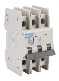
Gladiator miniature circuit breaker, 20A, 480Y / 277 VAC / 125 VDC, 3-pole, B curve, thermal magnetic, 10kA @ 480Y/277 VAC interrupting rating, 35mm DIN rail mount.
