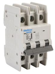
Gladiator miniature circuit breaker, 1A, 480Y / 277 VAC / 125 VDC, 3-pole, B curve, thermal magnetic, 10kA @ 480Y/277 VAC interrupting rating, 35mm DIN rail mount.
