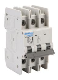
Gladiator miniature circuit breaker, 16A, 480Y / 277 VAC / 125 VDC, 3-pole, B curve, thermal magnetic, 10kA @ 480Y/277 VAC interrupting rating, 35mm DIN rail mount.
