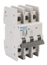
Gladiator miniature circuit breaker, 15A, 480Y / 277 VAC / 125 VDC, 3-pole, B curve, thermal magnetic, 10kA @ 480Y/277 VAC interrupting rating, 35mm DIN rail mount.
