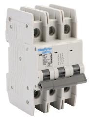
Gladiator miniature circuit breaker, 10A, 480Y / 277 VAC / 125 VDC, 3-pole, B curve, thermal magnetic, 10kA @ 480Y/277 VAC interrupting rating, 35mm DIN rail mount.
