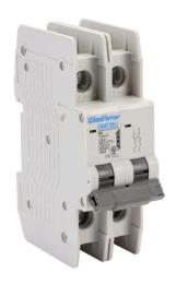
Gladiator miniature circuit breaker, 6A, 480Y / 277 VAC / 125 VDC, 2-pole, D curve, thermal magnetic, 10kA @ 480Y/277 VAC interrupting rating, 35mm DIN rail mount.
