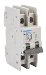
Gladiator miniature circuit breaker, 63A, 240 VAC / 125 VDC, 2-pole, D curve, thermal magnetic, 10kA @ 240 VAC interrupting rating, 35mm DIN rail mount.
