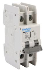
Gladiator miniature circuit breaker, 5A, 480Y / 277 VAC / 125 VDC, 2-pole, D curve, thermal magnetic, 10kA @ 480Y/277 VAC interrupting rating, 35mm DIN rail mount.
