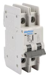
Gladiator miniature circuit breaker, 50A, 240 VAC / 125 VDC, 2-pole, D curve, thermal magnetic, 10kA @ 240 VAC interrupting rating, 35mm DIN rail mount.
