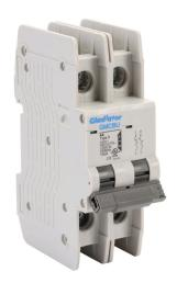
Gladiator miniature circuit breaker, 4A, 480Y / 277 VAC / 125 VDC, 2-pole, D curve, thermal magnetic, 10kA @ 480Y/277 VAC interrupting rating, 35mm DIN rail mount.
