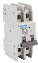
Gladiator miniature circuit breaker, 40A, 240 VAC / 125 VDC, 2-pole, D curve, thermal magnetic, 10kA @ 240 VAC interrupting rating, 35mm DIN rail mount.
