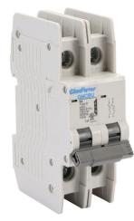
Gladiator miniature circuit breaker, 3A, 480Y / 277 VAC / 125 VDC, 2-pole, D curve, thermal magnetic, 10kA @ 480Y/277 VAC interrupting rating, 35mm DIN rail mount.
