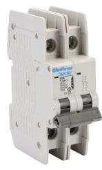
Gladiator miniature circuit breaker, 32A, 240 VAC / 125 VDC, 2-pole, D curve, thermal magnetic, 10kA @ 240 VAC interrupting rating, 35mm DIN rail mount.
