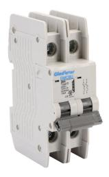
Gladiator miniature circuit breaker, 30A, 240 VAC / 125 VDC, 2-pole, D curve, thermal magnetic, 10kA @ 240 VAC interrupting rating, 35mm DIN rail mount.
