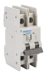
Gladiator miniature circuit breaker, 2A, 480Y / 277 VAC / 125 VDC, 2-pole, D curve, thermal magnetic, 10kA @ 480Y/277 VAC interrupting rating, 35mm DIN rail mount.
