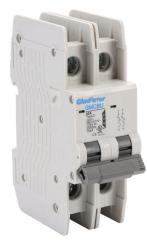
Gladiator miniature circuit breaker, 20A, 480Y / 277 VAC / 125 VDC, 2-pole, D curve, thermal magnetic, 10kA @ 480Y/277 VAC interrupting rating, 35mm DIN rail mount.
