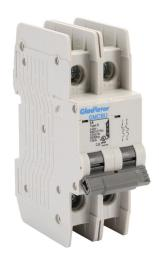
Gladiator miniature circuit breaker, 1A, 480Y / 277 VAC / 125 VDC, 2-pole, D curve, thermal magnetic, 10kA @ 480Y/277 VAC interrupting rating, 35mm DIN rail mount.
