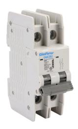
Gladiator miniature circuit breaker, 15A, 480Y / 277 VAC / 125 VDC, 2-pole, D curve, thermal magnetic, 10kA @ 480Y/277 VAC interrupting rating, 35mm DIN rail mount.
