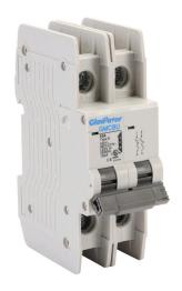
Gladiator miniature circuit breaker, 10A, 480Y / 277 VAC / 125 VDC, 2-pole, D curve, thermal magnetic, 10kA @ 480Y/277 VAC interrupting rating, 35mm DIN rail mount.
