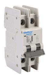
Gladiator miniature circuit breaker, 8A, 480Y / 277 VAC / 125 VDC, 2-pole, C curve, thermal magnetic, 10kA @ 480Y/277 VAC interrupting rating, 35mm DIN rail mount.
