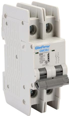
Gladiator miniature circuit breaker, 63A, 240 VAC / 125 VDC, 2-pole, C curve, thermal magnetic, 10kA @ 240 VAC interrupting rating, 35mm DIN rail mount.
