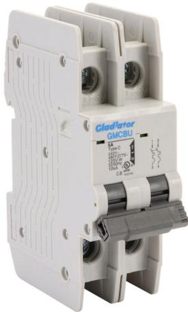
Gladiator miniature circuit breaker, 5A, 480Y / 277 VAC / 125 VDC, 2-pole, C curve, thermal magnetic, 10kA @ 480Y/277 VAC interrupting rating, 35mm DIN rail mount.
