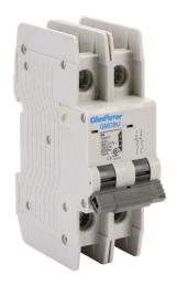
Gladiator miniature circuit breaker, 4A, 480Y / 277 VAC / 125 VDC, 2-pole, C curve, thermal magnetic, 10kA @ 480Y/277 VAC interrupting rating, 35mm DIN rail mount.
