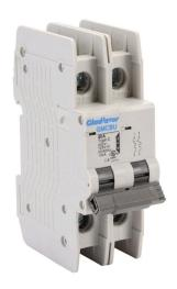
Gladiator miniature circuit breaker, 40A, 240 VAC / 125 VDC, 2-pole, C curve, thermal magnetic, 10kA @ 240 VAC interrupting rating, 35mm DIN rail mount.
