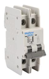
Gladiator miniature circuit breaker, 3A, 480Y / 277 VAC / 125 VDC, 2-pole, C curve, thermal magnetic, 10kA @ 480Y/277 VAC interrupting rating, 35mm DIN rail mount.
