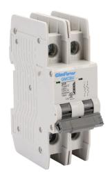
Gladiator miniature circuit breaker, 32A, 240 VAC / 125 VDC, 2-pole, C curve, thermal magnetic, 10kA @ 240 VAC interrupting rating, 35mm DIN rail mount.
