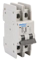
Gladiator miniature circuit breaker, 30A, 240 VAC / 125 VDC, 2-pole, C curve, thermal magnetic, 10kA @ 240 VAC interrupting rating, 35mm DIN rail mount.
