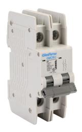
Gladiator miniature circuit breaker, 2A, 480Y / 277 VAC / 125 VDC, 2-pole, C curve, thermal magnetic, 10kA @ 480Y/277 VAC interrupting rating, 35mm DIN rail mount.
