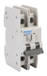
Gladiator miniature circuit breaker, 25A, 480Y / 277 VAC / 125 VDC, 2-pole, C curve, thermal magnetic, 10kA @ 480Y/277 VAC interrupting rating, 35mm DIN rail mount.
