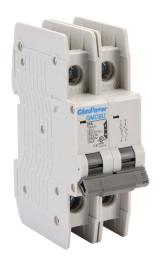
Gladiator miniature circuit breaker, 20A, 480Y / 277 VAC / 125 VDC, 2-pole, C curve, thermal magnetic, 10kA @ 480Y/277 VAC interrupting rating, 35mm DIN rail mount.
