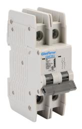
Gladiator miniature circuit breaker, 1A, 480Y / 277 VAC / 125 VDC, 2-pole, C curve, thermal magnetic, 10kA @ 480Y/277 VAC interrupting rating, 35mm DIN rail mount.
