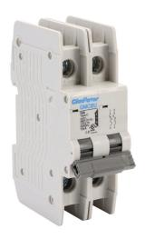
Gladiator miniature circuit breaker, 16A, 480Y / 277 VAC / 125 VDC, 2-pole, C curve, thermal magnetic, 10kA @ 480Y/277 VAC interrupting rating, 35mm DIN rail mount.
