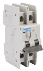
Gladiator miniature circuit breaker, 15A, 480Y / 277 VAC / 125 VDC, 2-pole, C curve, thermal magnetic, 10kA @ 480Y/277 VAC interrupting rating, 35mm DIN rail mount.
