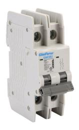
Gladiator miniature circuit breaker, 10A, 480Y / 277 VAC / 125 VDC, 2-pole, C curve, thermal magnetic, 10kA @ 480Y/277 VAC interrupting rating, 35mm DIN rail mount.
