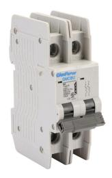
Gladiator miniature circuit breaker, 8A, 480Y / 277 VAC / 125 VDC, 2-pole, B curve, thermal magnetic, 10kA @ 480Y/277 VAC interrupting rating, 35mm DIN rail mount.
