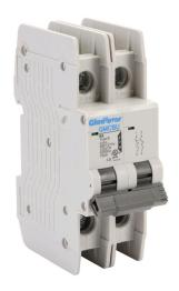
Gladiator miniature circuit breaker, 6A, 480Y / 277 VAC / 125 VDC, 2-pole, B curve, thermal magnetic, 10kA @ 480Y/277 VAC interrupting rating, 35mm DIN rail mount.
