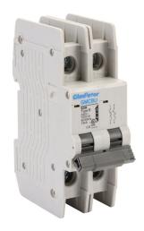
Gladiator miniature circuit breaker, 63A, 240 VAC / 125 VDC, 2-pole, B curve, thermal magnetic, 10kA @ 240 VAC interrupting rating, 35mm DIN rail mount.
