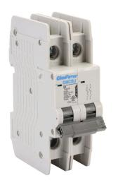
Gladiator miniature circuit breaker, 5A, 480Y / 277 VAC / 125 VDC, 2-pole, B curve, thermal magnetic, 10kA @ 480Y/277 VAC interrupting rating, 35mm DIN rail mount.
