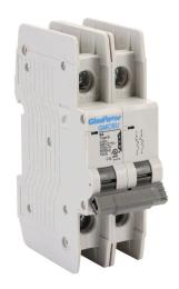
Gladiator miniature circuit breaker, 4A, 480Y / 277 VAC / 125 VDC, 2-pole, B curve, thermal magnetic, 10kA @ 480Y/277 VAC interrupting rating, 35mm DIN rail mount.
