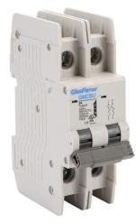
Gladiator miniature circuit breaker, 3A, 480Y / 277 VAC / 125 VDC, 2-pole, B curve, thermal magnetic, 10kA @ 480Y/277 VAC interrupting rating, 35mm DIN rail mount.
