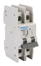
Gladiator miniature circuit breaker, 32A, 240 VAC / 125 VDC, 2-pole, B curve, thermal magnetic, 10kA @ 240 VAC interrupting rating, 35mm DIN rail mount.
