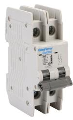
Gladiator miniature circuit breaker, 30A, 240 VAC / 125 VDC, 2-pole, B curve, thermal magnetic, 10kA @ 240 VAC interrupting rating, 35mm DIN rail mount.
