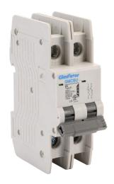
Gladiator miniature circuit breaker, 2A, 480Y / 277 VAC / 125 VDC, 2-pole, B curve, thermal magnetic, 10kA @ 480Y/277 VAC interrupting rating, 35mm DIN rail mount.
