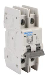
Gladiator miniature circuit breaker, 25A, 480Y / 277 VAC / 125 VDC, 2-pole, B curve, thermal magnetic, 10kA @ 480Y/277 VAC interrupting rating, 35mm DIN rail mount.
